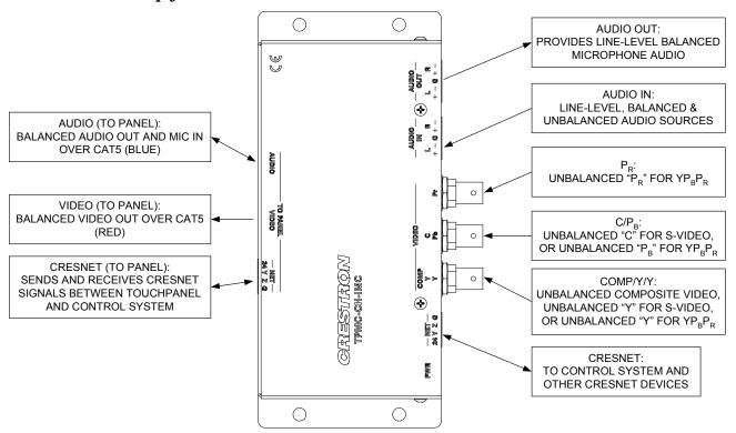
A triamese cable that is included with the touchpanel has an RJ-45 connector with a blue cover to match the blue label on the TPMC-CH-IMC and an RJ-45 connector with a red cover to match the red label on the TPMC-CH-IMC. The cable also has a 4-position miniterminal block connector for making a network connection between the touchpanel and the TPMC-CH-IMC.
